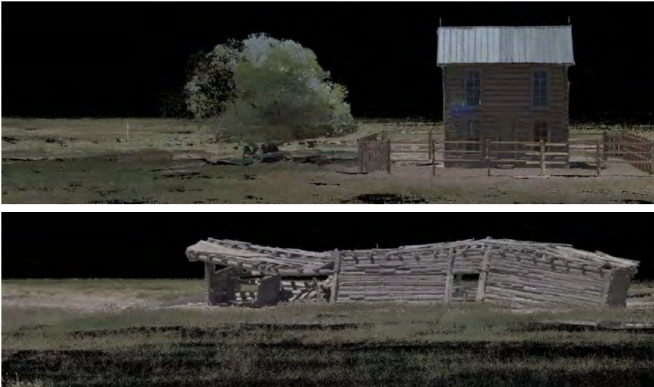
■ Using modern technology to document the past. The team developed two virtual tours and several “images,” as seen above, of the Trujillo Homestead sites developed from the LiDAR scans. (Center for Preservation Research/University of Colorado Denver)
