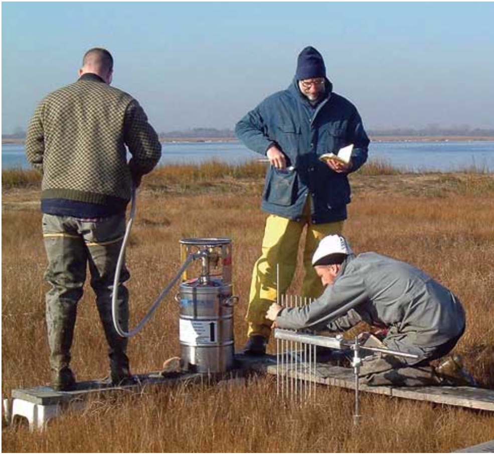
Figure 1. Investigators examine measuring pins in the rod-type surface elevation table to discern changes in overall marsh elevation. A third scientist prepares to freeze a marsh core sample using liquid nitrogen.
